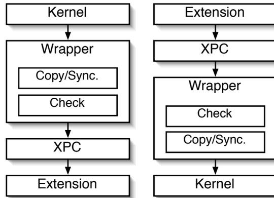
Fig. 4. Control flow of extension and kernel wrappers.
