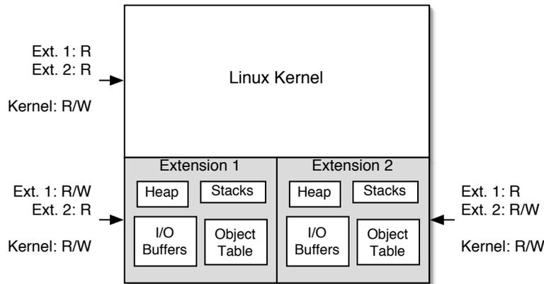
Fig. 3. Protection of the kernel address space.
